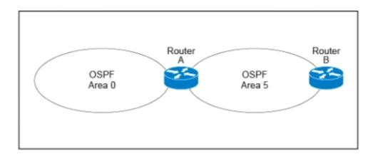
A customer runs OSPF with Area 5 between its aggregation router and an internal router When a network change occurs in the backbone. Area 5 starts having connectivity issues due to the SPF algorithm recalculating an abnormal number of times in Area 5 You are tasked to redesign this network to increase resiliency on the customer network with the caveat that Router B does not support the stub area How can you accomplish this task\*?
