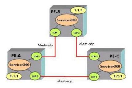
A new router named PE-D is to be directly connected to PE-C and is required to be added to the existing VPLS 300. The design requires the least amount of signaling, the least amount of configuration changes for existing sites and the new site has to have access to all existing sites. How should the new site be added to VPLS 300?
