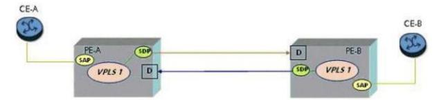
CE-A sends frames with 2 tags. If the SAP on PE-A is "sap 1/1/1:1 .\*" and the SAP on PE-B is "sap 1/1/1:100.200" how many tags will there be on the frame when it egresses from the SAP on PE-B?
