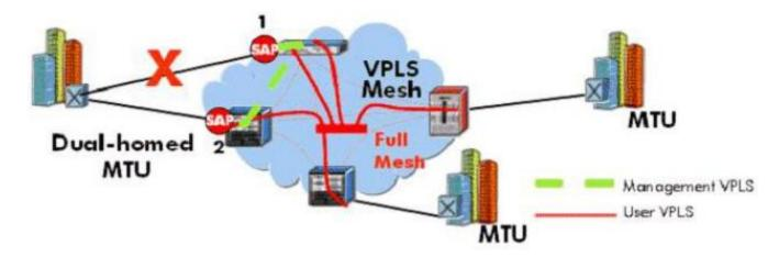
In the diagram below, SAP 1 is put into the blocking state as a result of the spanning tree protocol. What will occur in the VPLS instance if SAP 2 goes down and SAP 1 transitions to the forwarding state? Select the most accurate statement.
