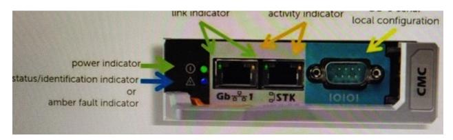
An administrator has a standalone M1000e chassis with only a single CMC module. The Cat6 cable is plugged into the Ethernet port closed to the DG-9 connector. The power indicator light is lit but the administrator is unable to access the CMC module.
