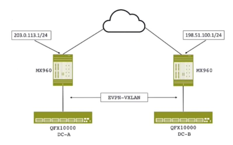
You are designing a Data Center Interconnect to transport VXLAN traffic between DC-A and DC-B
