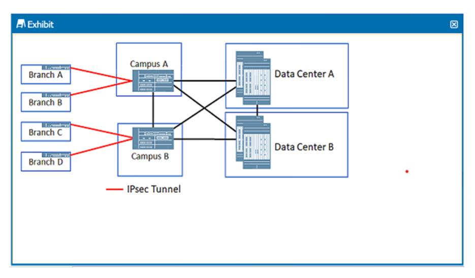
In the 3-tier VPN design shown in the exhibit, which function are the Campus A and Campus B SRX Series devices performing?
