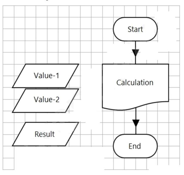
This is the Main Page of a simple process which calls the 'Calculation' Page before completing.
