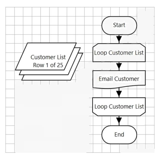
The 'Loop Customer List' loop is configured to loop through the 'Customer List' Collection.
