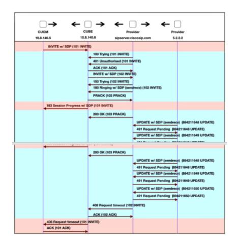
A Cisco Unified Border Element continues to send 180/183 with the required: 100rel header to Cisco UCM. and the call eventually disconnects How is the issue resolved?
