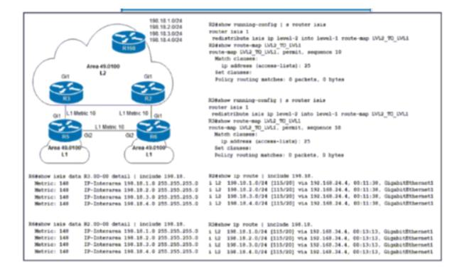
Routers R2 and R3 are Level 1/Level 2 IS-IS routers that redistribute 198 18.x.x/24 prefixes to routers R5 and R6 In the Level 1 area R2 Is to be the preferred router for all redistributed prefixes in the Level 1 are
