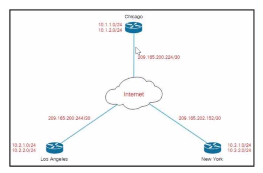
Company XYZ must design a DMVPN tunnel between the three sites Chicago is going to act as the NHS and the company wants DMVPN to detect peer endpoint failures Which technology should be used m the design?
