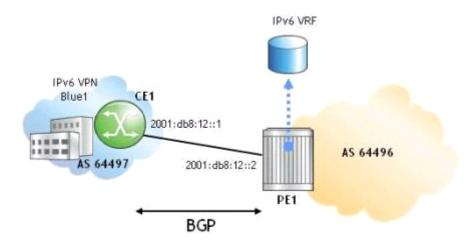
Part of a 6VPE deployment is shown. Which of the following is the correct configuration and context on router CE1 for a BGP peering session with 6VPE1?
