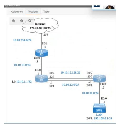
IP connectivity and OSPF are preconfigured on all devices where necessary. Do not make any changes to the IP addressing or OSPF. The company policy uses connected interfaces and next hops when configuring static routes except for load balancing or redundancy without floating static. Connectivity must be established between subnet 172.20.20.128/25 on the Internet and the LAN at 192.168.0.0/24 connected to SW1:
