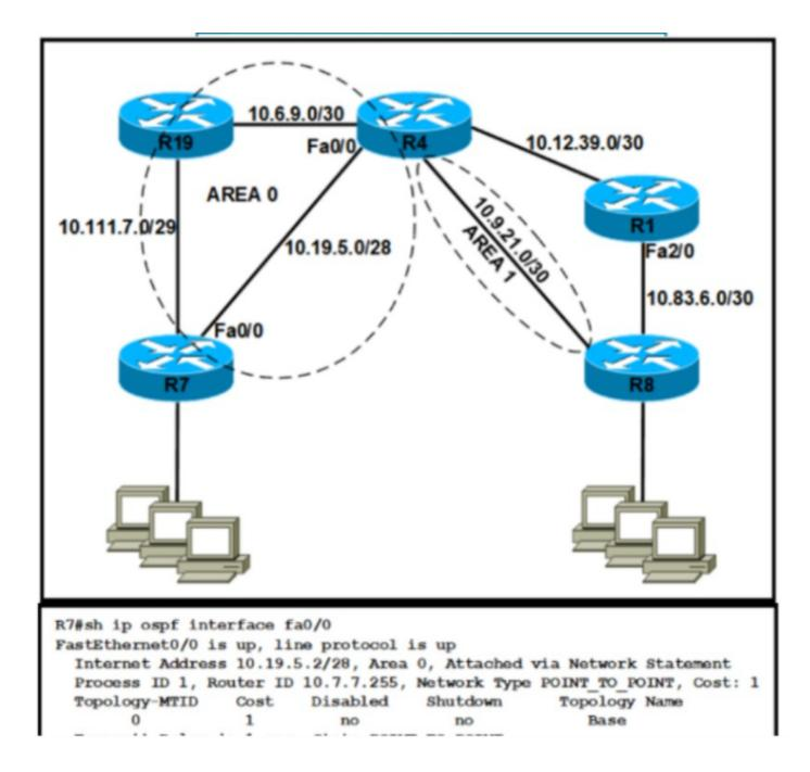
Refer to the exhibit. Router R4 is configured correctly with default OSPF values. A network engineer configured R7 for OSPF. R7 must not be elected as a DR for the segment between R4-R7. The adjacency between R4 and R7 failed to form. Which configuration resolves the issue?
