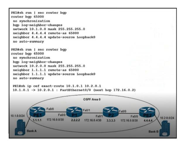
Refer to the exhibit. Network connectivity between bank A and bank B has been lost Users at bank A and bank B are able to successfully reach their directly connected PE routers. All routers in OSPF area 0 are correctly advertising and learning routing updates. Which action resolves the issue?
