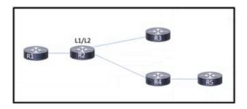
Refer to the exhibit Reuters R2. R3, R4 and R5 all reside in the same area, with R1 in a different area R3 is overutilized and the engineer wants to reduce its CPU load The engineer configured router R4 to summarize routes that it receives from R5. but R3 is still receiving all of the R5 routes. Which action resolves the issue?
