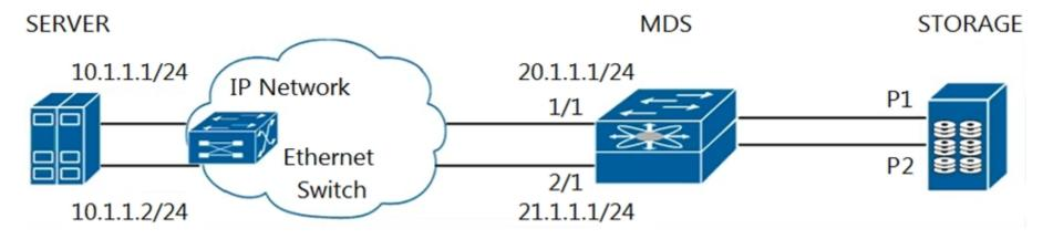
A high-availability setup for iSCSI is designed with the host running iSCSI multipath software. Each IP storage port on the MDS switch exports the same two Fibre Channel target ports with different iSCSI target names.
