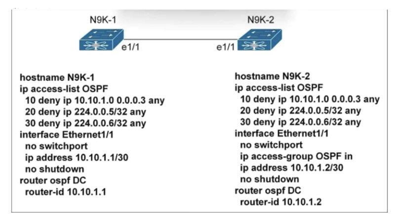
A client reports that the routing protocol neighborship fails to start between two Cisco Nexus switches, N9K-1 and N9K-2. Which action resolves the issue?
