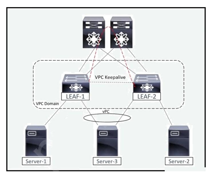
An engineer is troubleshooting the connectivity between Server-1 and Server-2. Which action resolves the connectivity issue?
