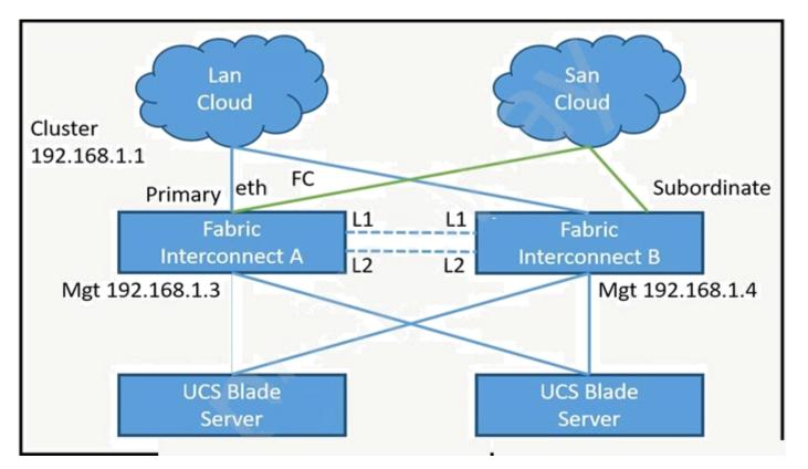
A network engineer finds one of the fabric interconnects offline when connecting L1 and L2 ports on both fabric interconnects. Which action resolves the issue?
