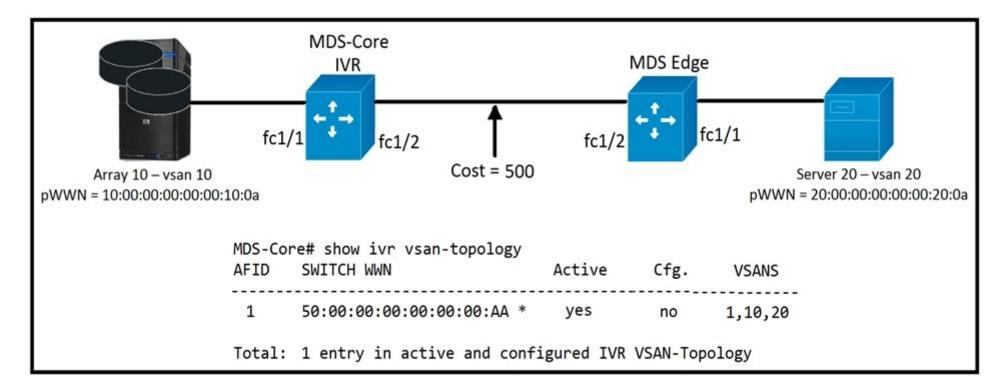
An engineer is configuring Inter-VSAN routing for two Cisco MDS switches. The FSPF cost between the switches is 500, and the Cisco MDS core virtualizes an IVR NAT domain as shown. Which statement about the topology is correct?
