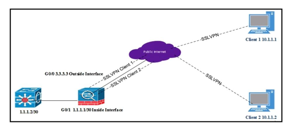
All internal clients behind the ASA are port address translated to the public outside interface that has an IP address of 3.3.3.3. Client 1 and client 2 have established successful SSL VPN connections to the ASA. What must be implemented so that "3.3.3.3" is returned from a browser search on the IP address?
