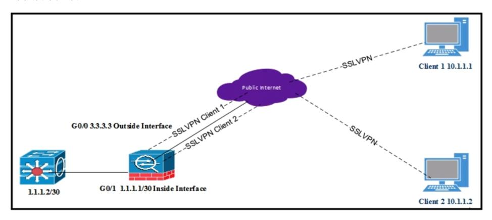
All internal clients behind the ASA are port address translated to the public outside interface that has an IP address of 3.3.3.3. Client 1 and client 2 have established successful SSL VPN connections to the ASA. What must be implemented so that "3.3.3.3" is returned from
