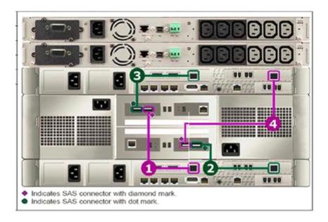
Based on the XtremIO naming convention, what is the correct name for the source and the destination port for number 1?
