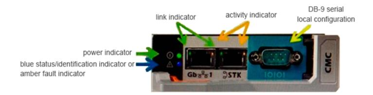
An administrator has a standalone M1000e chassis with only a single CMC module. The CAT6 cable is plugged into the Ethernet port closest to the DB-9 connector. The power indicator light is lit but the administrator is unable to access the CMC module.
