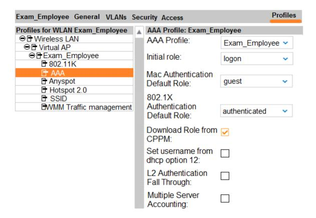
The exhibit shows the AAA profile for a WLAN on an Aruba solution. This WLAN uses 802.1X to authenticate users to a RADIUS server. A user successfully authenticates with 802.1X, but the RADIUS server does not send a role assignment.
