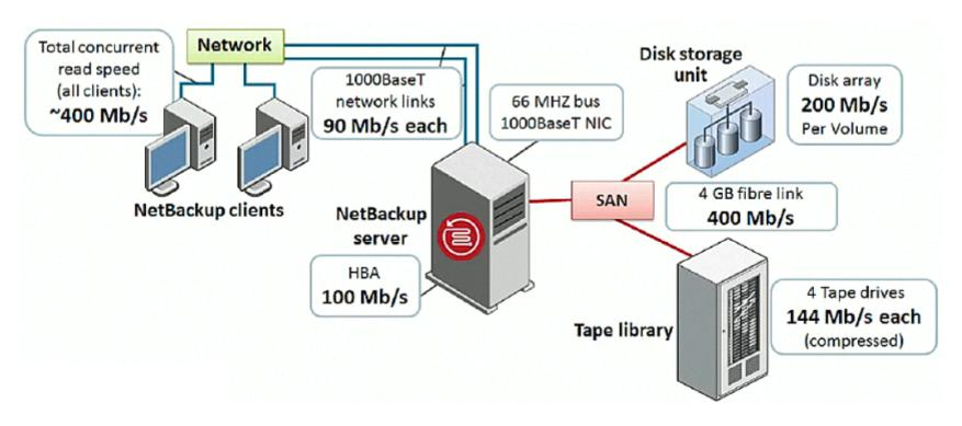
An administrator is analyzing the NetBackup environment with a view to optimizing backup performance. The environment has been mapped according to the diagram shown below.
