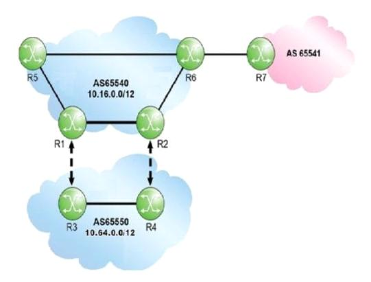
AS 65550 owns CIDR block 10.64.0.0/12. Router R6 advertises the aggregate 10.64.0.0/12 to AS 65541 with "as-set" enabled. Which of the following is TRUE regarding the aggregate route received by router R7?
