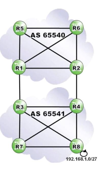
Router R2 receives a route to 192.168.1.0/27 from router R4, and sets the local preference to 110. Router R1 receives a route to 192.168.1.0/27 from router R3, and sets the local preference to 80. Both ASs have a full iBGP mesh. What path does traffic destined to 192.168.1.0/27 take from router R1?
