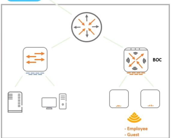
A 7008 Branch Office Controller (BOC) is deployed in a remote office behind a core router. This core does not support 802.1q encapsulation. The Mobility Controller (MC) is the gateway for two tunneling mode SSIDs, as shown in the exhibit.
