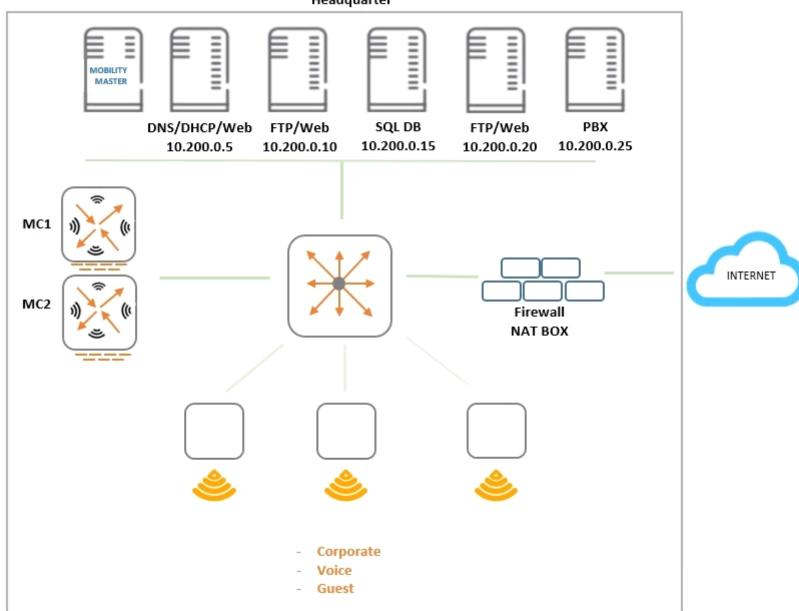
An organization provides WiFi access through a corporate SSID with an Aruba Mobility Master (MM) - Mobility Controller (MC) network that includes PEF functions. The organization wants to have a single firewall policy configured and applied to the employee role.
