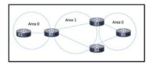
Refer to the exhibit. A network engineer just replaced five routers on this OSPF network. When the routing protocol is brought up, R5 cannot reach routes that originate on R1. The engineer verified that all connected links have established neighbor relationships. R5 reaches routes originating on R3 and R4. Which action resolves the issue?
