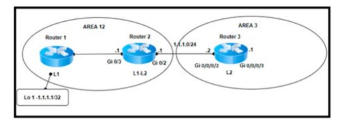
Refer to the exhibit. A network engineer configured three new PE routers to expand the network. The new routers run in the IS-IS routing protocol and reside in the data center in the same exchange as the existing routers. However, the network is now experiencing suboptimal routing. The Layer 2 configuration and VLANs are configured correctly to provide segregation between networks, but the Level 1 routes are not being converted to Level 2 routes. Which action resolves the issue?
