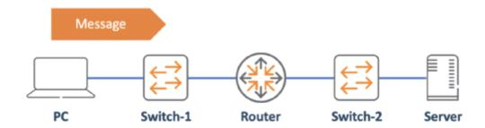
The PC is sending a message to the server. Which devices have performed Layer 2 encapsulation by the time the message arrives at the server? (Select two.)
