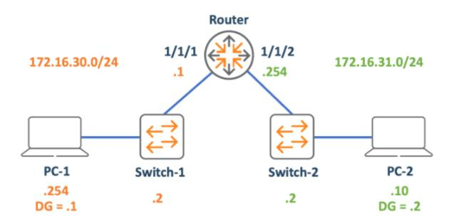
The PCs are not able to successfully establish bidirectional communication. What change must you deploy to enable the communication between PC-1 and PC-2?
