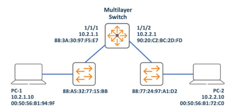
PC-1 is sending a packet to PC-2. What are the Layer 2 and Layer 3 source addresses of the message when it is received by PC-2? (Select two.)
