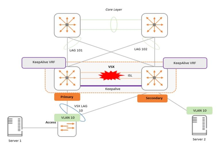
Two AOS-CX switches are configured for VSX at the access layer, where servers attached to them. An SVI interface is configured for VLAN 10 and serves as the default gateway for VLAN 10. The ISL link between the switches fails, but the keepalive interface functions. Active gateway has been configured on the switches.
