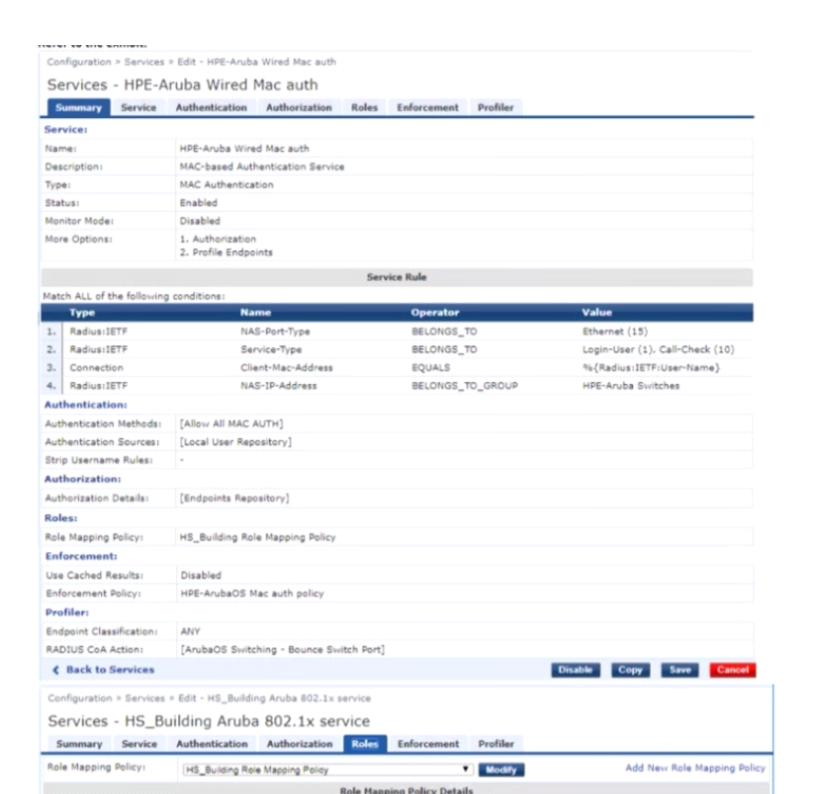
You configured the Wired MAC - Auth service enforcement conditions with the Endpoint profiling data When mac-auth based clients connect to the network, ClearPass assigns Deny access profile. The customer has sent you the above screenshots How would you resolve the issue?
