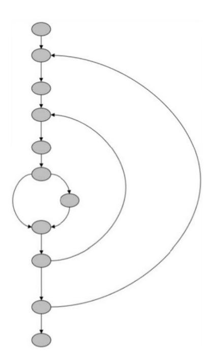
The control flow represents a software component of a car navigation system. Within the project the maximum cyclomatic complexity to be allowed is set at 5.
