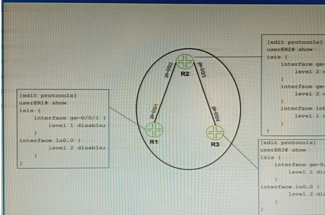
Referring to the exhibit, which two configuration changes must you apply for packets to reach from R1 to R3 using IS-IS? (Choose two.)
