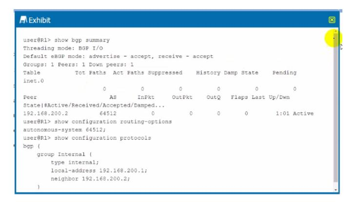
Referring to the exhibit, internal BGP between R1 and R2 is not establishing.
