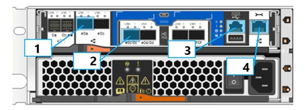
Referring to the numbers shown in the exhibit, which port on an AFF A220 controller is used as port e0M in ONTAP?
