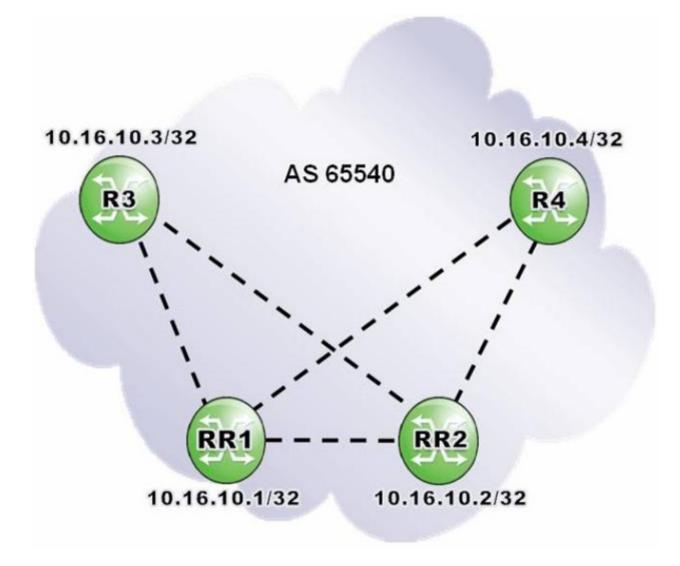
Routers RR1 are RR2 are redundant route reflectors for clients R3 and R4. Which of the following is a valid configuration on router RR1?
