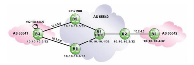
Router R1 is a route reflector with clients R2, R5 and R6. Prefixes advertised by router R5 have a local preference of 200. Router R3 advertises the prefix 192.168.1.0/27 to routers R5 and R6. Assuming that router R6 is configured with "advertise-external", what is the expected output of "show router bgp routes" when executed on router R1?
