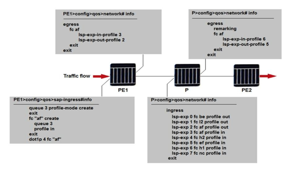
Traffic corresponding to a layer-3 VPN arrives at router PE1 marked with a dot1p value of 4. The SDP carrying the traffic uses an MPLS transport tunnel. Given the policies applied on the routers in the diagram, what is the EXP value of packets arriving at router PE2?
