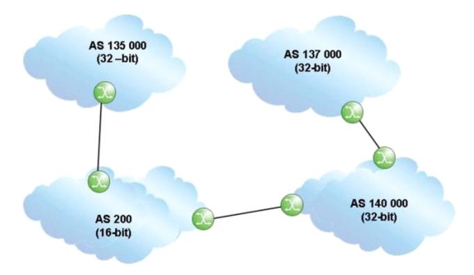
An update travels from AS 137000 to AS 135000, traversing both 32-bit and 16-bit AS Paths.
