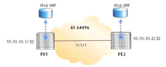
The two PEs are providing 6VPE and IPv4 VPRNs. The core network is IPv4/MPLS. Which of the following is the BGP family configuration for the MP-BPG on the PEs?
