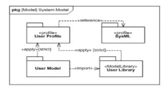
The User Profile extends SysML with two new stereotypes of Block Hardware and Software.
