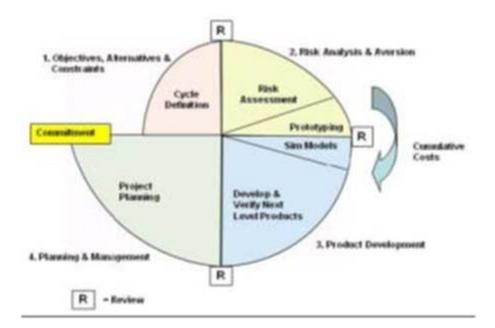
The diagram is of the \_\_\_\_\_ Development Model.
