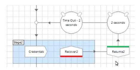
The developer of this flow found that writing some credentials to the target application sometimes failed with an exception even though the element exists on the screen. He found that simply catching the exception, waiting for 2 seconds and then retrying fixed the problem.
