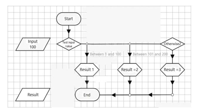
The Process flow is intended to test the value of the Input data item to determine if it falls within a range of numbers, and then assign a value as an output. The number ranges are defined as between 1 to 100, between 101 to 200, and anything outside these ranges.
