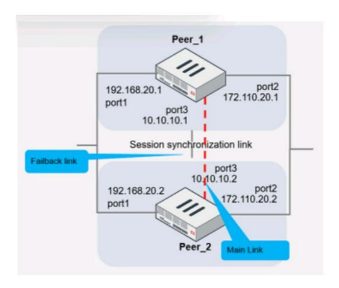
The main link directly connects the two FortiGate devices and is configured using the set
