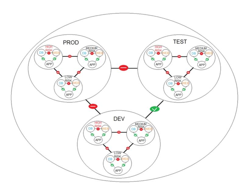
A financial company is adopting micro-services with the intent of simplifying network security. An NSX-T architect is proposing a NSX-T Data Center micro-segmentation logical design. The architect has created a diagram to share with the customer.
